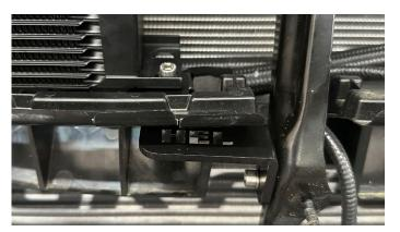
**8.** Attach the top bracket to the existing bolt holes. The right side uses the bonnet latch bracket.
