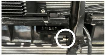
**10.** When re-attaching the radiator shroud, you will need to trim the plastic back. This enables full air flow for the cooler, cut along the white line.
