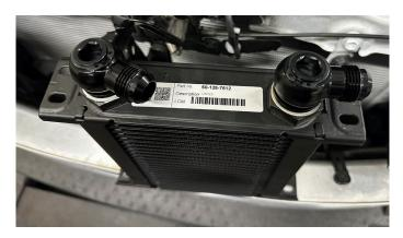
**6.** Install the supplied upper bracket to the cooler including bolts, o-rings and nuts.
