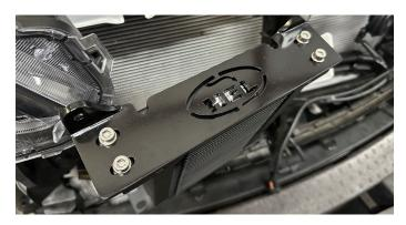
7. Install the bottom bracket with the supplied hardware. Attach the hoses, being careful to support the banjo's whilst tightening.
