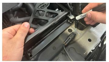
**4.** Carefully drill out the newly marked hole. Take care to not drill to deep through the whole. (using a small length of wood will protect the underside of the drilling)
