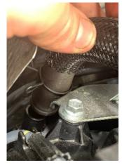
**8.** Re-using the factory retaining clip from the 90 degree breather hose end, install the longer silicone hose to the intake pipe.
