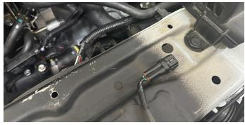
**5.** Attach the catch can to the bracket using the supplied hardware. Attach the bracket & catch can assembly to the newly drilled hole.
