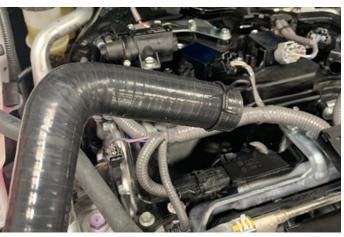
**9.** Install the remaining hose to the valve cover port.
