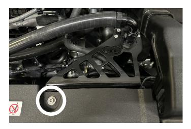
**7.** Remove the engine cover. Locate the valve cover breather hose and disconnect it at both ends.
