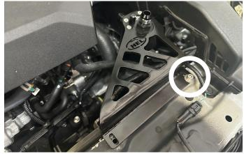
**6.** Re-attach the front tray, and install the bolt back through the left side of the catch can bracket. Attach both the hoses to the catch can, and route them out to the left side, as seen in the image. (90° top port, 150° side port)
